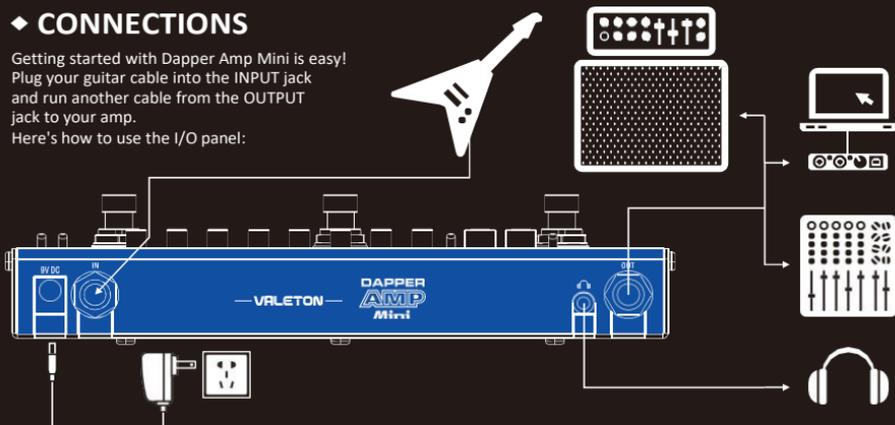
Note: 1. If Dapper Amp Mini sounds harsh or weird when connecting to the input jack on your amp, try connecting to the amp's FX Loop return jack.
